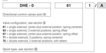
= NBR **PE** = FKM BT Series number = HNBR Voltage code, see section 5
