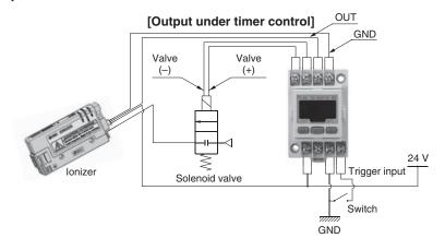
■Solenoid valves up to 24 VDC (4 W) etc. are controllable.
