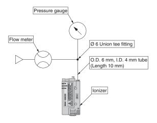
Fig. 1: Flow rate characteristics measuring circuit
