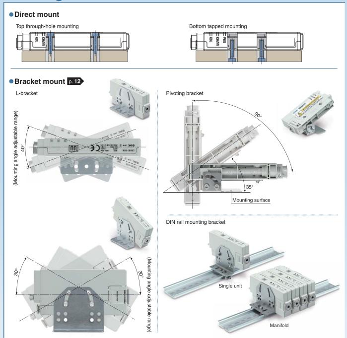
· The L-bracket and the DIN rail mounting bracket can be used with the manifold.
