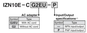
\*1 Select the same input/output specification as the ionizer.
