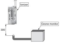
Fig. 2: Ozone condensation measuring circuit
