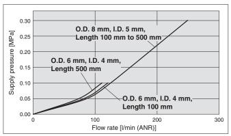
\* When a pressure above each line is used, the maintenance warning function may work and turn on the LED. Refer to "Cautions when using the IZN10E-11□□□-□ female threads for piping" on page 10.
