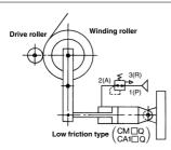
Pressure is kept steady, responding rapidly to the position change of the piston in the cylinder.
