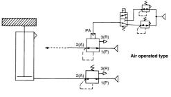
Pressure changes during cylinder actuation are suppressed, balancing the cylinder in both static and dynamic conditions.
