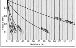
3. Relief time from an arbitrary pressure [Example] VEX 1500 lowers 2000 L tank from 0.4 MPa to 0.1 MPa:
