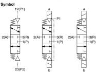
Air operated External pilot solenoid Internal pilot solenoid
