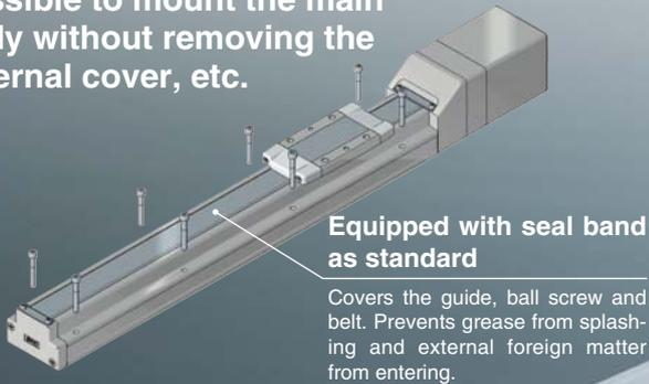
Equipped with seal band
